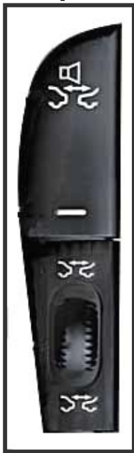
Console switches (S46/8)
