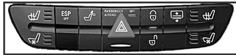
Upper Control Panel (N72/1)
